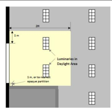
**Daylight Extension Factor (DEF):** factor to manually calculate the daylight area on floor plates. It is to be multiplied by the head height of windows. It is dependent on orientation and glazing VLT, shading devices adjacent to it and building location.
