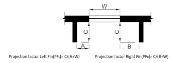
**Projection Factor, overhang and side fin:** average of ratio projection factor for overhang only and projection factor of side fin only.
