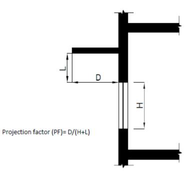
**Projection factor, side fin:** the ratio of the horizontal depth of the external shading projection to the distance from the window jamb to the farthest point of the external shading projection, in consistent units.
