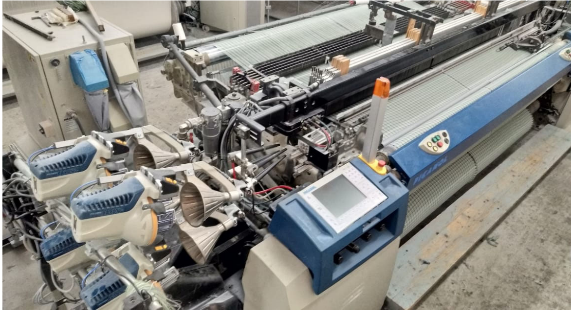
Airjet loom fitted with Electronic 4 Colour Feeder at Tamil Nadu Textile Corporation Limited, Coimbatore
