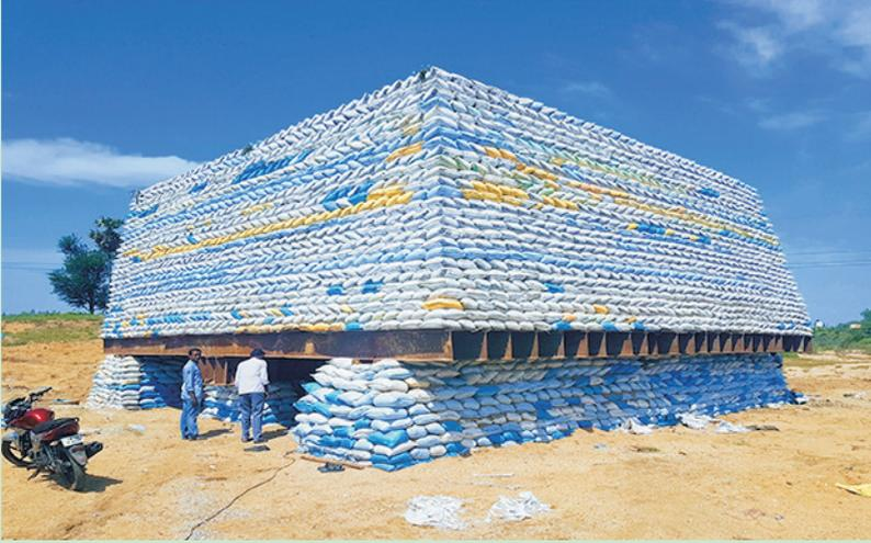
**Pile load test to assess the strength of Bridge Pile**
